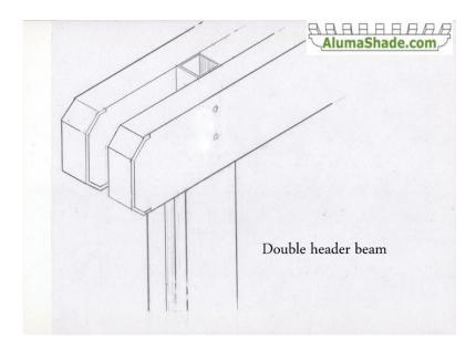
The double header beam is good for greater spans between posts of the patio covers. It also works well with fiberglass columns.
