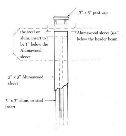
Installation configuration for a double header beam Laguna lattice cover
