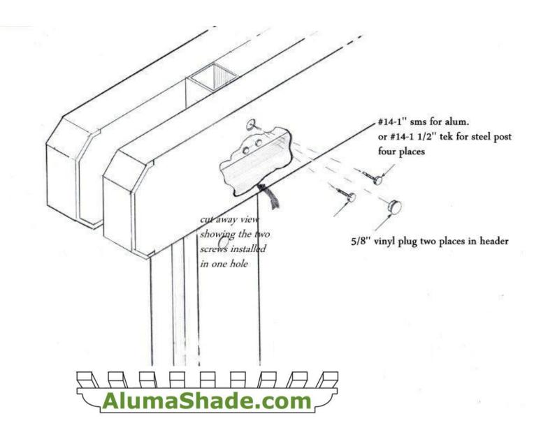
Drill the 5/8" holes in the header beams in the center of the post, two inches down from the top and bottom of the header beam. Put two screws in each hole, and then install the vinyl screw plugs.
