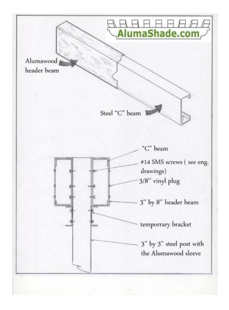
When installing C-beams make sure the back of the C-beam is against the post.
